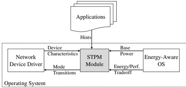
Figure 3: STPM software architecture
