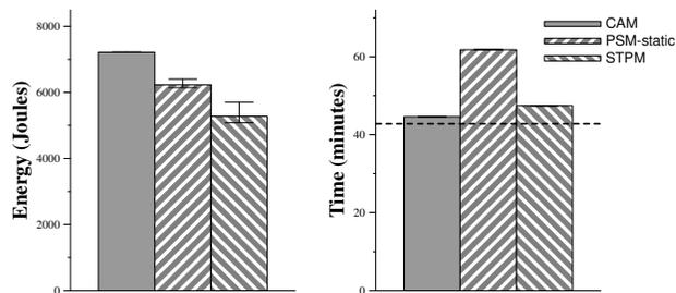
These graphs show the time and energy needed to execute NFS operations using a Orinoco Silver 802.11b card. These results can be compared to those in figure 15 for the Cisco Aironet 350 card. It is not possible to disable the Orinoco card, nor does it support an adaptive power saving mode. Each bar shows the mean of three trials—the error bars show the value of the minimum and maximum trial.
