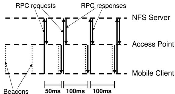
Figure 2: RPC delays due to power management
