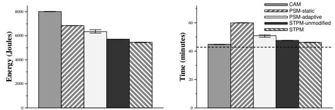
These graphs show how the hinting module with STPM performs compared to other power management policies. Each bar shows the mean of three trials—the error bars show the value of the minimum and maximum trial.
