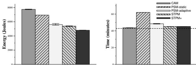
These graphs show how the choice of power management policy affects the time and energy needed to execute NFS operations. Each bar shows the mean of three trials—the error bars show the value of the minimum and maximum trial.
