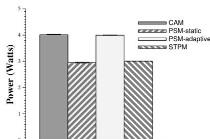
These graphs show how the choice of power management policy affects the power used to play streaming audio on an iPAQ using XMMS. Each bar shows the mean of three trials—the error bars show the value of the minimum and maximum trial.
