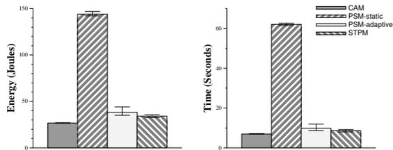
These graphs show how the choice of power management policy affects the time and energy needed to run remote X applications. The rightmost graph shows the time to start the Gnumeric application running on the server with the display on the iPAQ client, load a spreadsheet, and close the application—the leftmost graph shows the total energy expended. Each bar shows the mean of three trials—the error bars show the value of the minimum and maximum trial.
